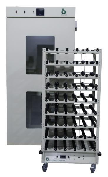
Bellco's Roll-In Incubators are built to accommodate large-scale roller apparatus setups with ease. Designed for uniform temperature distribution and optimal airflow, these units maintain a consistent environment for high-yield cell culture. With durable stainless-steel interiors, easy-access doors, and reliable controls, Bellco incubators make scaling up as simple as rolling in.
